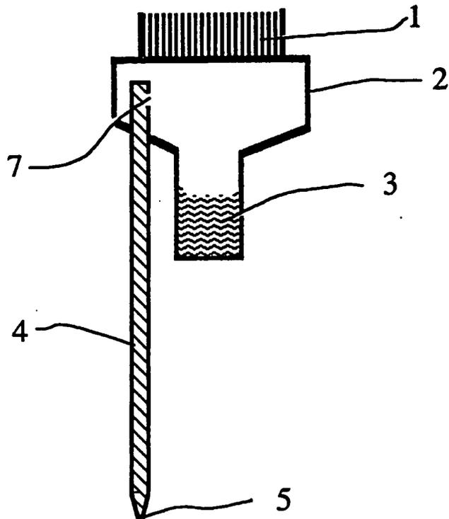
**Apparatus (cuvette) for taking up and storing liquids and for carrying out optical measurements**
